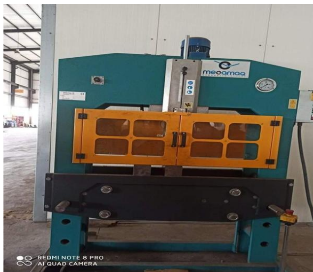
Figure II.19: presse hydraulique de 50 tonnes
