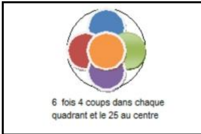
Figure III.6 : Compactage des couches
