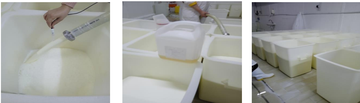
Figure 10 : Cuve de coagulation.
