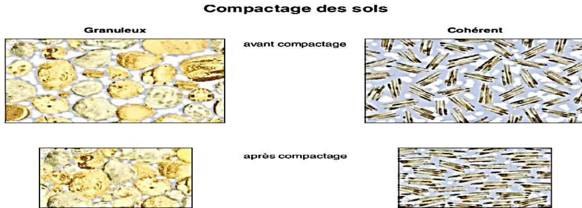
Figure 1.IV. Compactage des sols.
