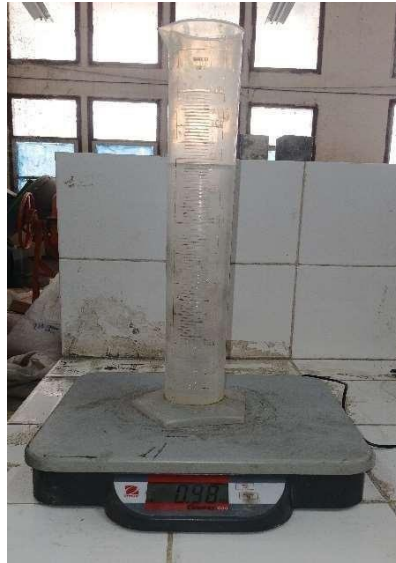
Figure III-2 :L'eau de gâchage.
