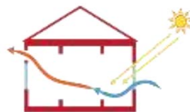
Figure 140. Ventilation naturelle (file:///C:/Users/CLIENT/Downloads/Ms.Arc.
