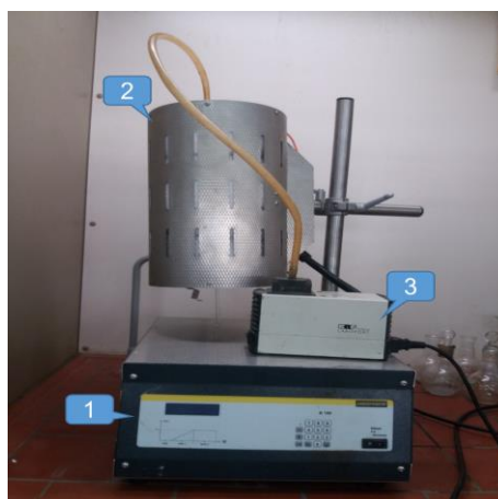
Figure II.6 : Four tubulaire NOBERTHERM
