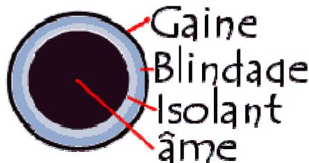
Figure-I-15- Câble coaxial
