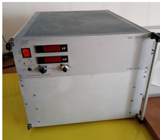
Figure III.3 Source Haute Tension continue
