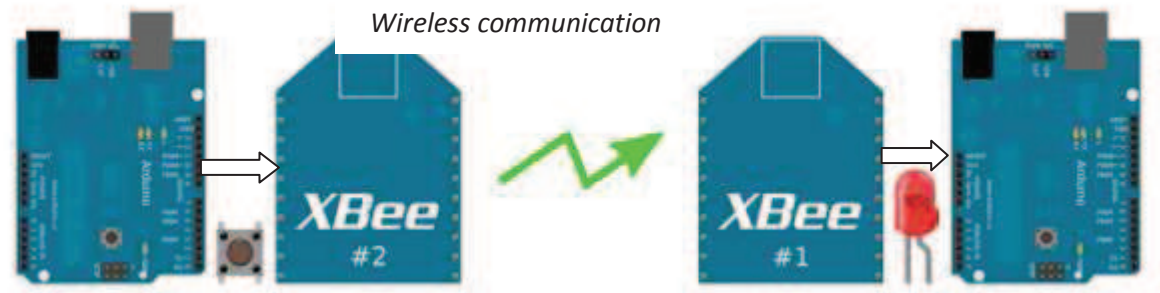
Figure-3.17-: shows two Arduinos communicating using Xbee
