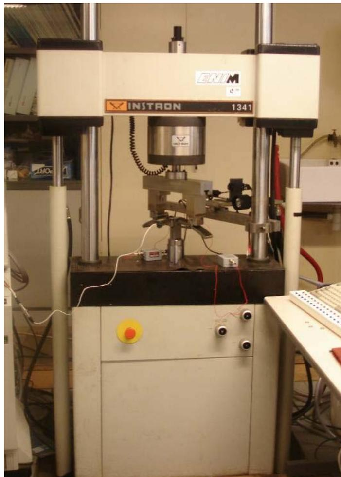
**Figure II.9 :** Machine de traction/compression INSTRON 1341.
