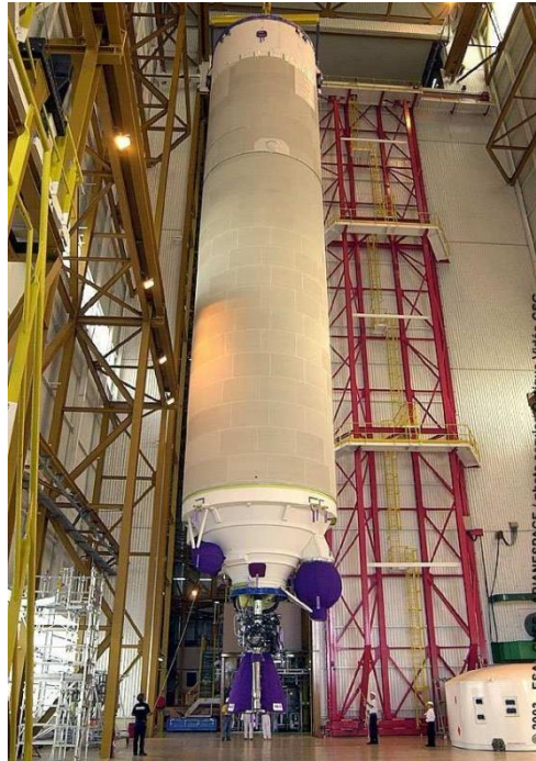
Figure I.6: Etage Principale Cryotechnique.
