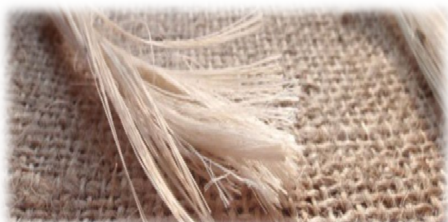
Figure II.3 : Fibres de jute. [30]
