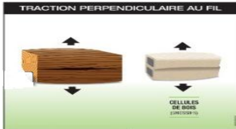
Figure I.23 : Contrainte de rupture de traction transversale.
