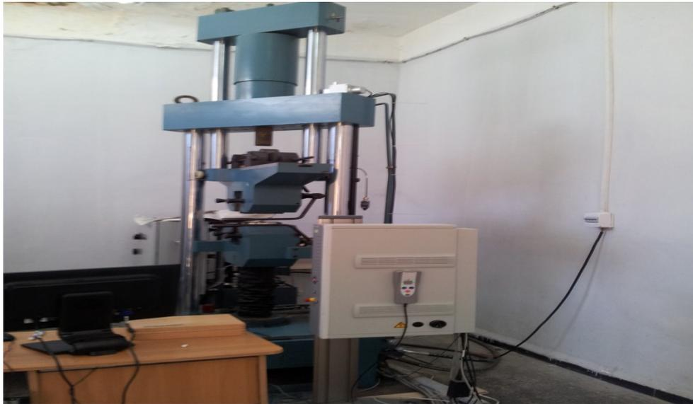
Figure III.6 : Machine universelle de traction zwick roell (600kN)
