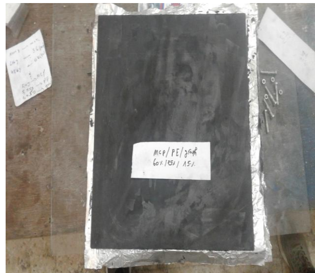
d) plaque de 60%MCP, 25%perlite, 15% graphite
