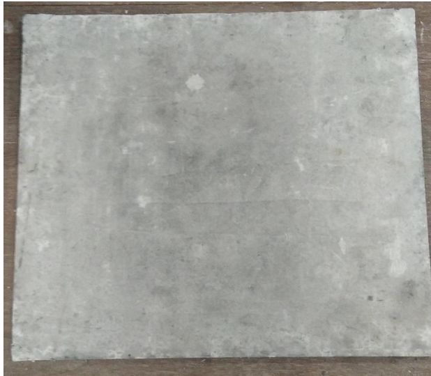
a) Plaque de 60 %MCP, 40% Perlite (Sans graphite)
