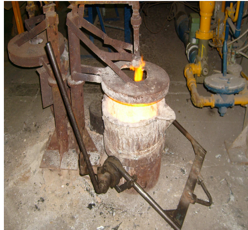
Figure II.1.4 - Poche de coulée
