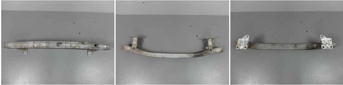
Figure 3.21 – RENFORCEMENT BARRE DE PARE CHOCS .(www.eurofrance)
