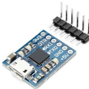
FIGURE 4.3 – Tranceiver USB to UART.
