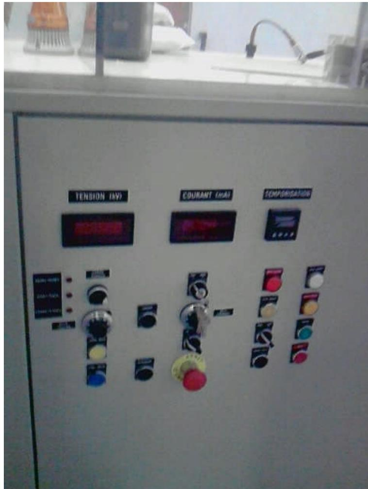
Figure IV.8. Source de tension alternative.
