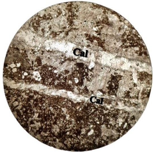
Figure 45: Calcite fine en veinule tardive. (LM), LPA. G.x10)
