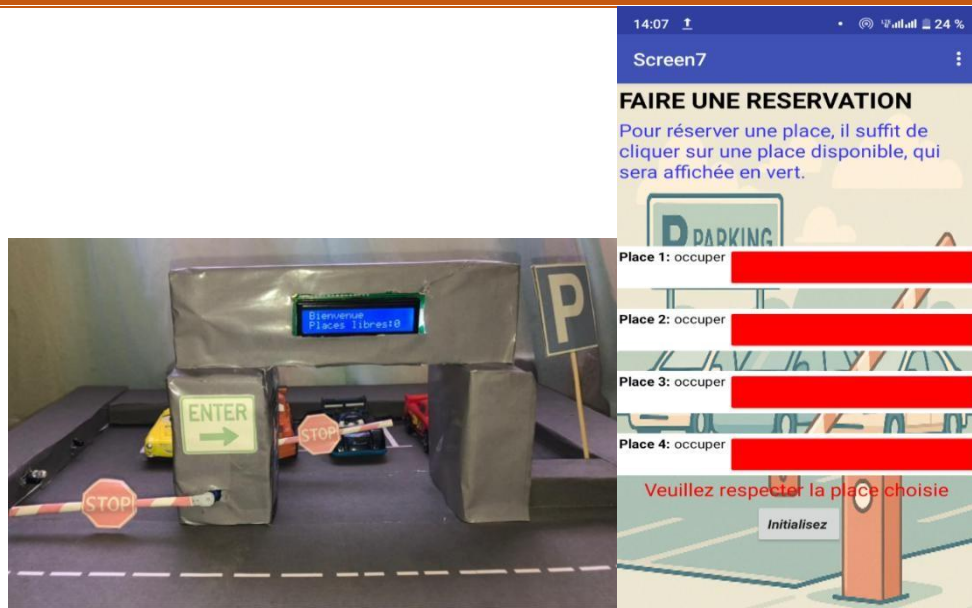
Figure III.51 : Affichage maquette et application — Parking plein.
