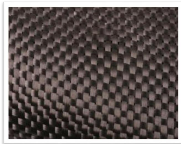
Figure I.6: Tissu de fibres de carbone.
