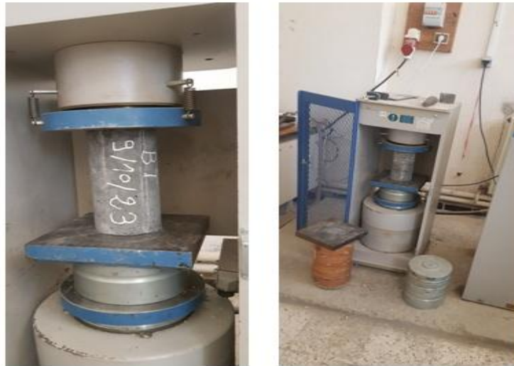
Figure III.6 : Essai mécanique de compression.
