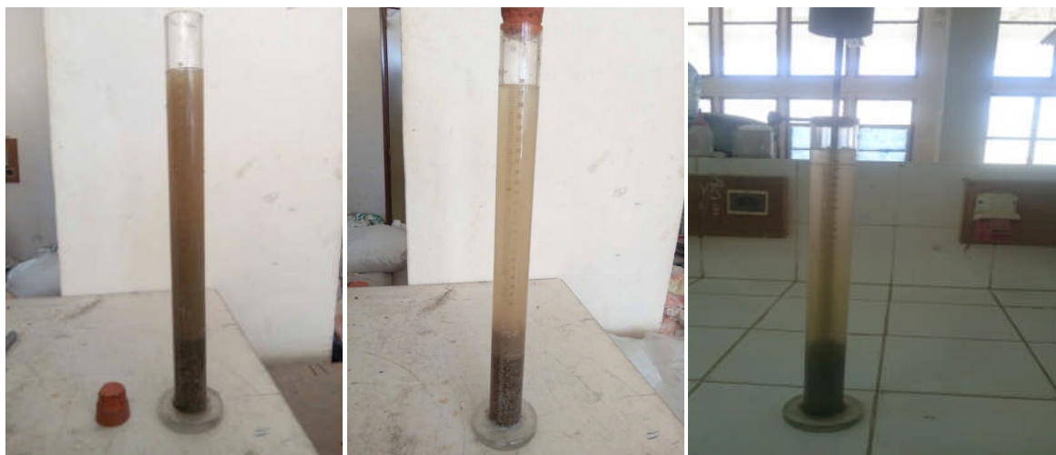
Figure IV-7: Equivalent de sable
