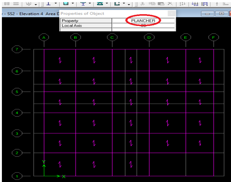
Figure 4-16 Affectation des plancher
