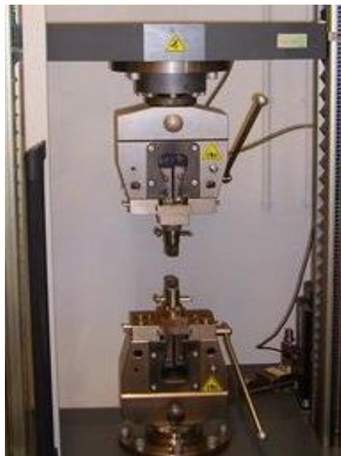
**Figure I.6 :** Machine de traction [2]
