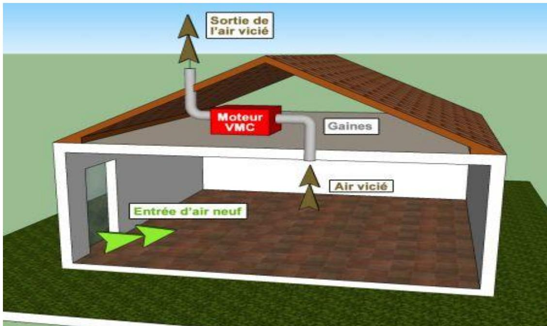
Figure I-13 : VMC simple flux
