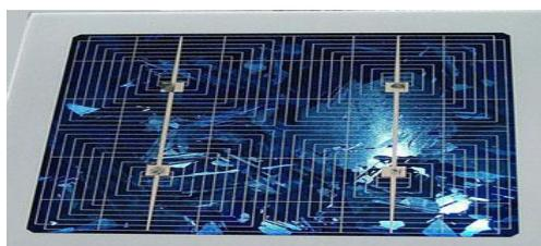
**Figure I-6: Cellules poly cristallines [2]**
