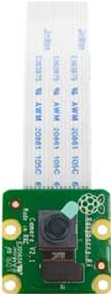
FIGURE 3.3 – raspberry pi camera module 2
