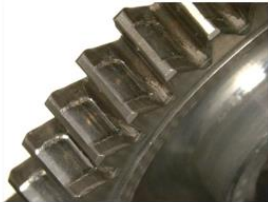
Figure II-3 : Usure due au frottement.
