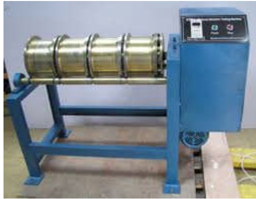
Figure VIII-8 : Essai Micro Deval
