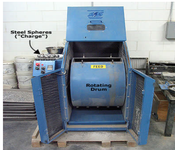
Figure VIII-7 : Essai Los Angeles
