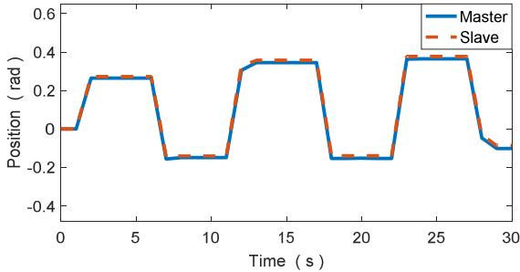
Fig. 6. Motion tracking behavior with PID controllers.
