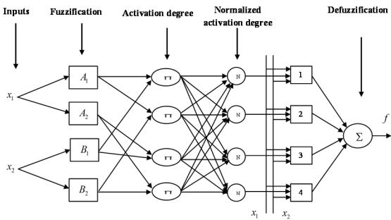
Fig. 2. ANFIS controller architecture.
