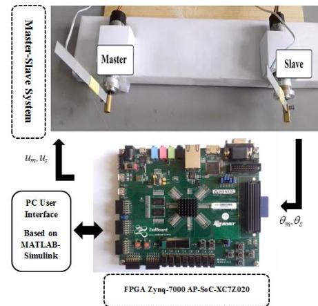
Fig. 5. The master-slave experimental system.
