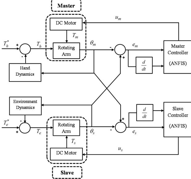
Fig. 1. Position-position control architecture with ANFIS controller.
