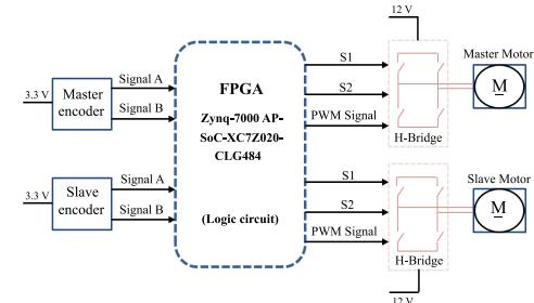
Fig. 4. Electronic circuit of the teleoperation system.
