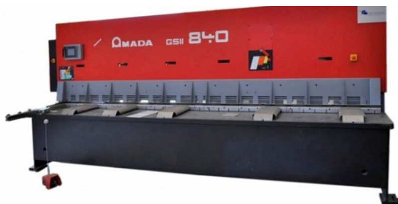
Figure I-9: Guillotine AMADA GSII 840.
