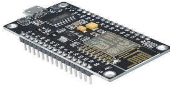
Figure I.8: Module WI-FI ESP8266.
