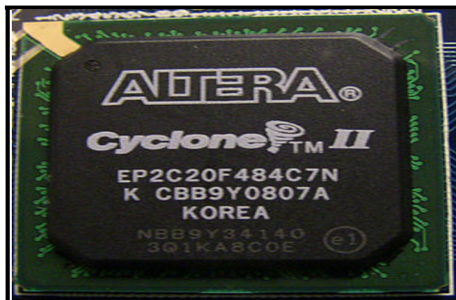
Figure II-11 : Structure externe de FPGA cyclone-II
