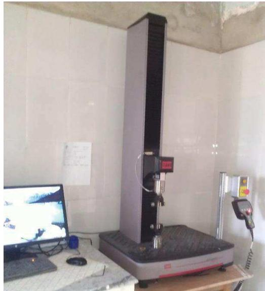
Figure III.23. Machine de traction
