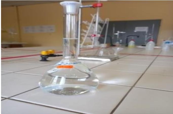
Figure 9 : Fiole contenant le diluant (solution de NaOH 0.1 M)
