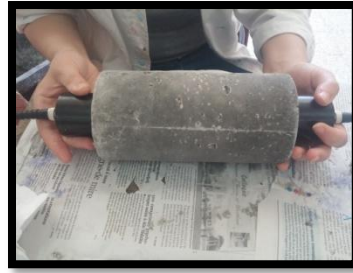
Figure II.7. Essai à ultrason transmission directe.
