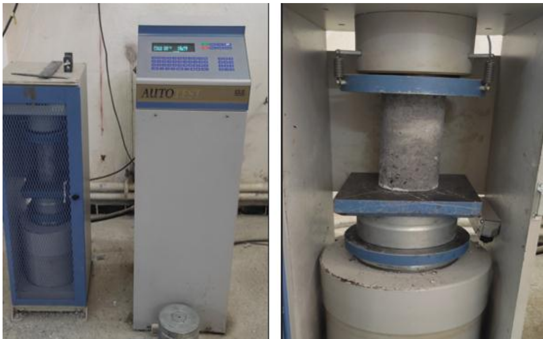
Figure III-7: la machine de compression.
