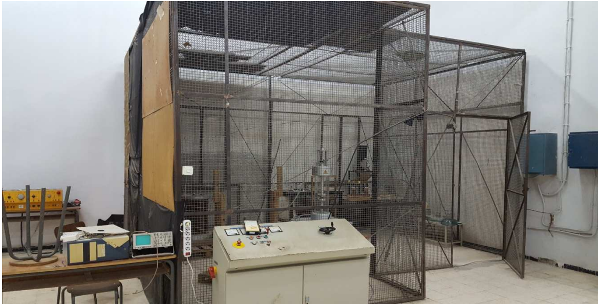
Figure III.4 Cage Faraday de laboratoire haute tension
