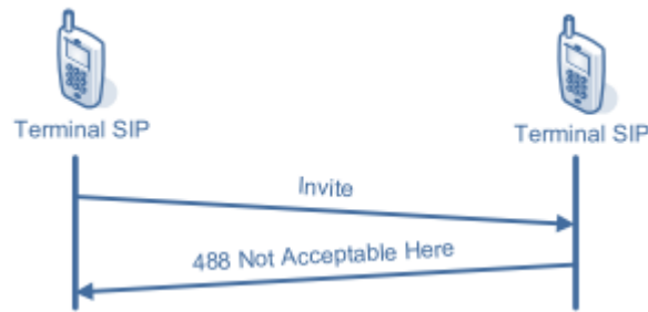
Figure II.16 : Modification d'une communication.
