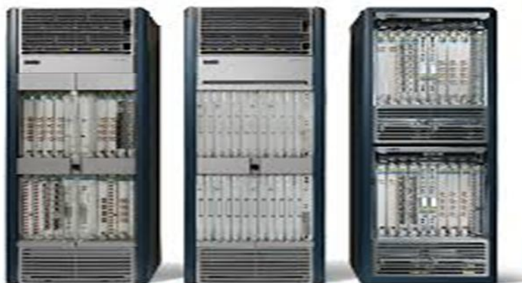
Fig.12. Equipment MSAN (Huawei UA5000)
